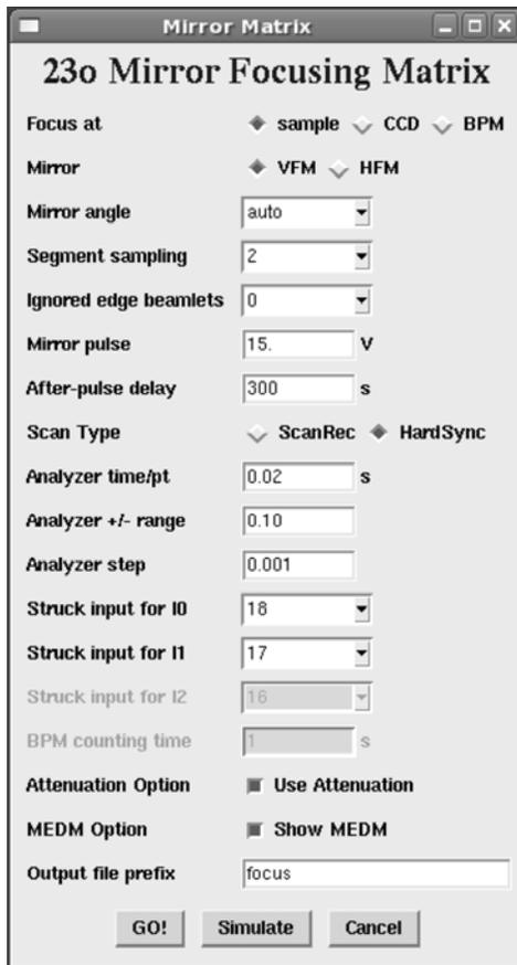
**Figure 2** – The tcl/tk GUI used for setting up automated collection of the matrix data.
