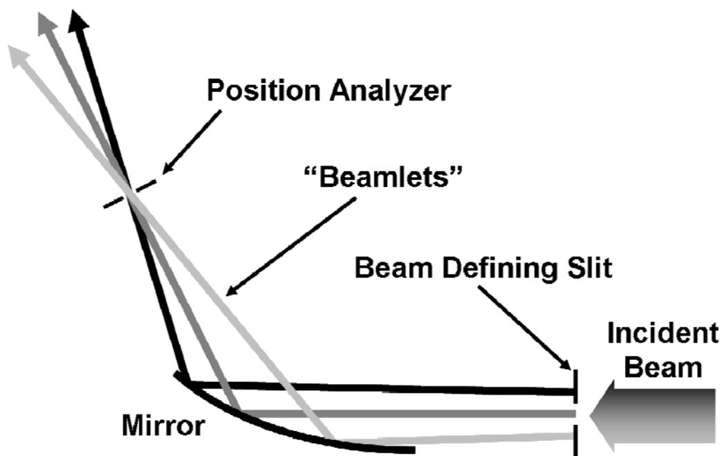
**Figure 1** – A schematic representation of the technique for assembling the interaction matrix.
