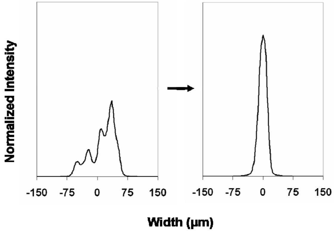
**Figure 3** – The matrix inversion technique efficiently focuses the beam in just a single step.
